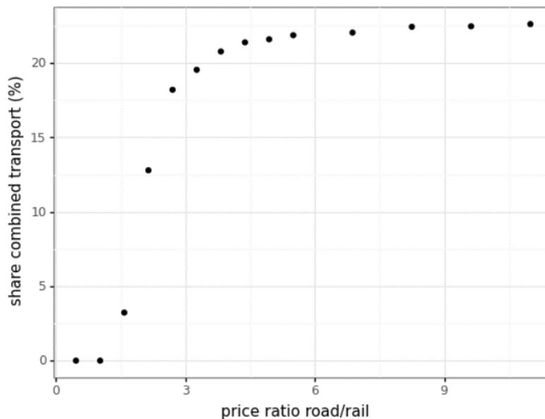
The results indicate the potential impact of autonomous driving technology and resulting reductions in road operation costs on the attractiveness of combined transport. To present an attractive alternative from the users' point of view, the combined transport mode requires that cost rates per container-kilometer for the road system are at least 3 times higher compared to the rail system.
