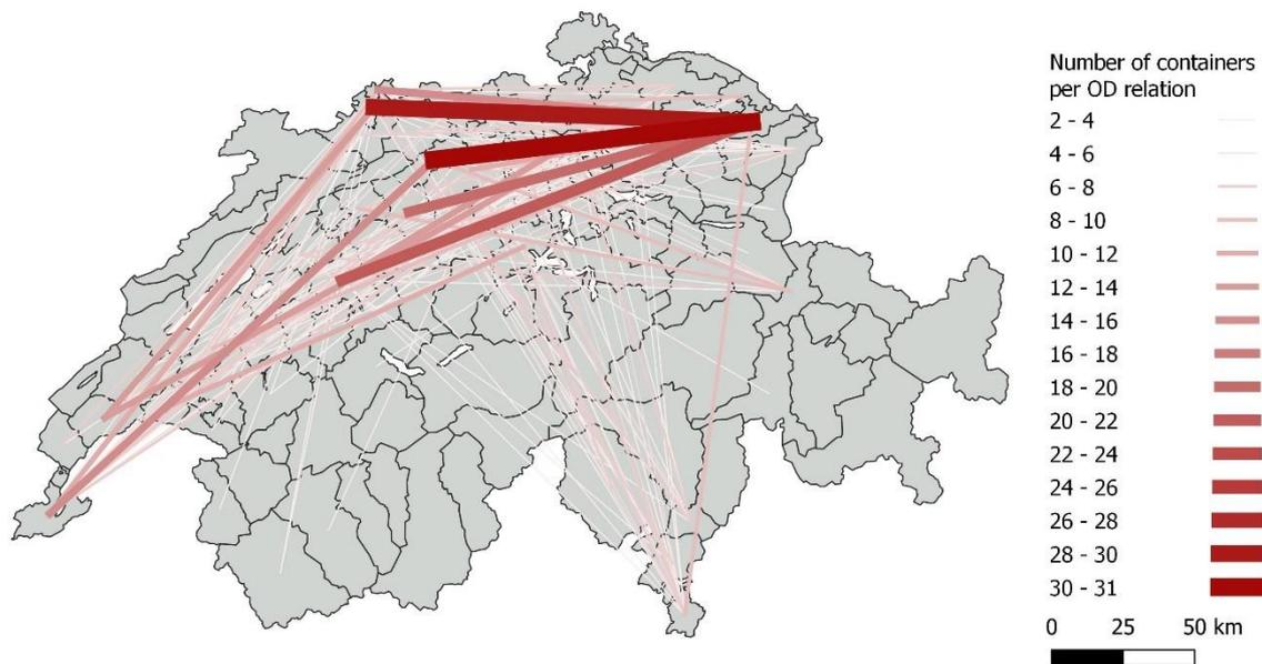
Most containers are routed through the rail network using a single cargo line. Only 14% of all container agents have a transfer and are loaded from one train to another one.
