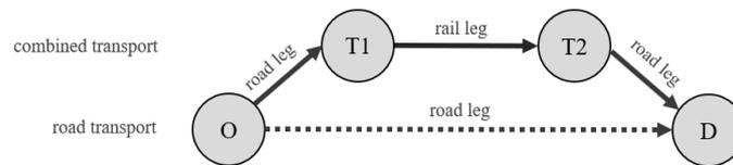
The agent's generalized cost function contains shipping relevant cost components, including departure and arrival time constraints related to the supply chain (see later in Sec. 2.3).
