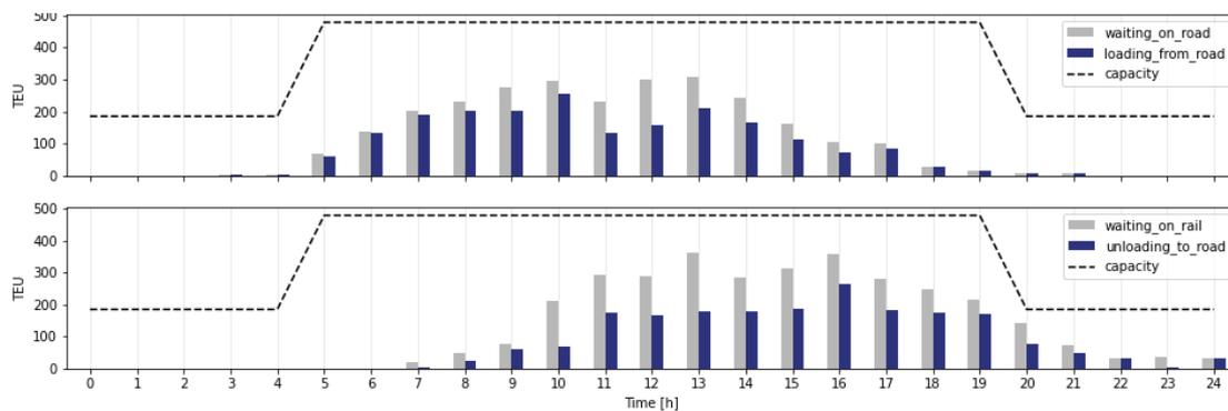
The bar height in Fig. 9 shows the number of **containers on trains** leaving a terminal (upper plot) and entering a terminal (lower plot) per time of day and summed up across all terminals.
