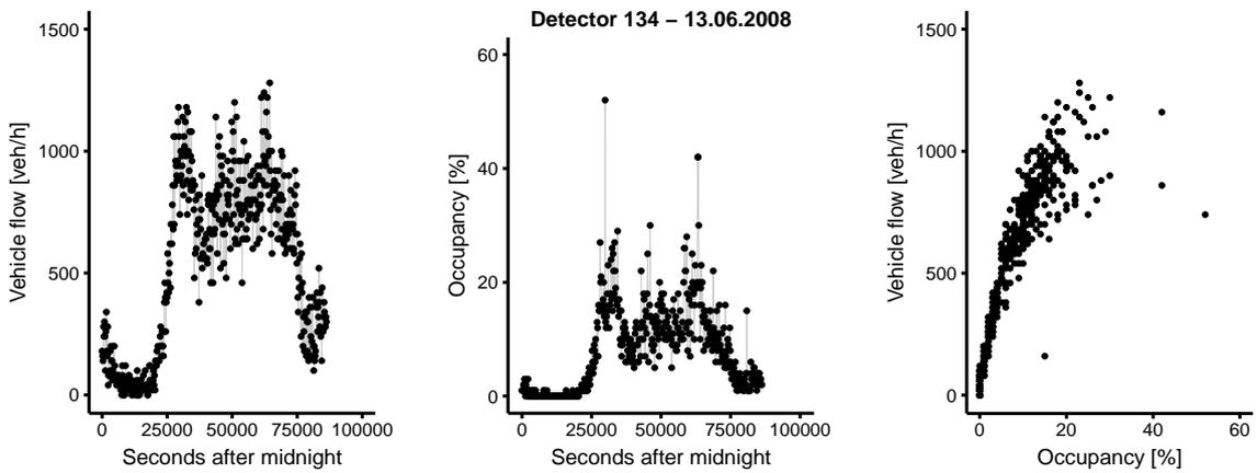
(d) Scatter plots of a loop detectors in Graz, Austria, with some observations considered as false and, subsequently removed from the sample.
