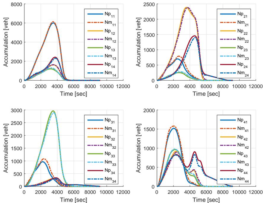
Figure 6: Vehicle accumulations  $n_i$  for the plant (blue lines) and the convex model without OD information (dashed black lines) when applied for 12 steps of prediction ( $k_m = 12k_c$ ).
