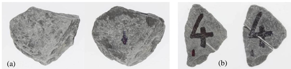
Particle breakage is the dissection of grains into parts occurring generally under high stress levels, while abrasion is a phenomenon whereby very small particles disintegrate from the grain surface, independent of stress level (Indraratna et al., 2011). According to Indraratna et al. (2009), aggregate breakage under rail loading is a complex mechanism initiating at inter-particle contacts, followed by breakage of the weaker particles upon further loading.
