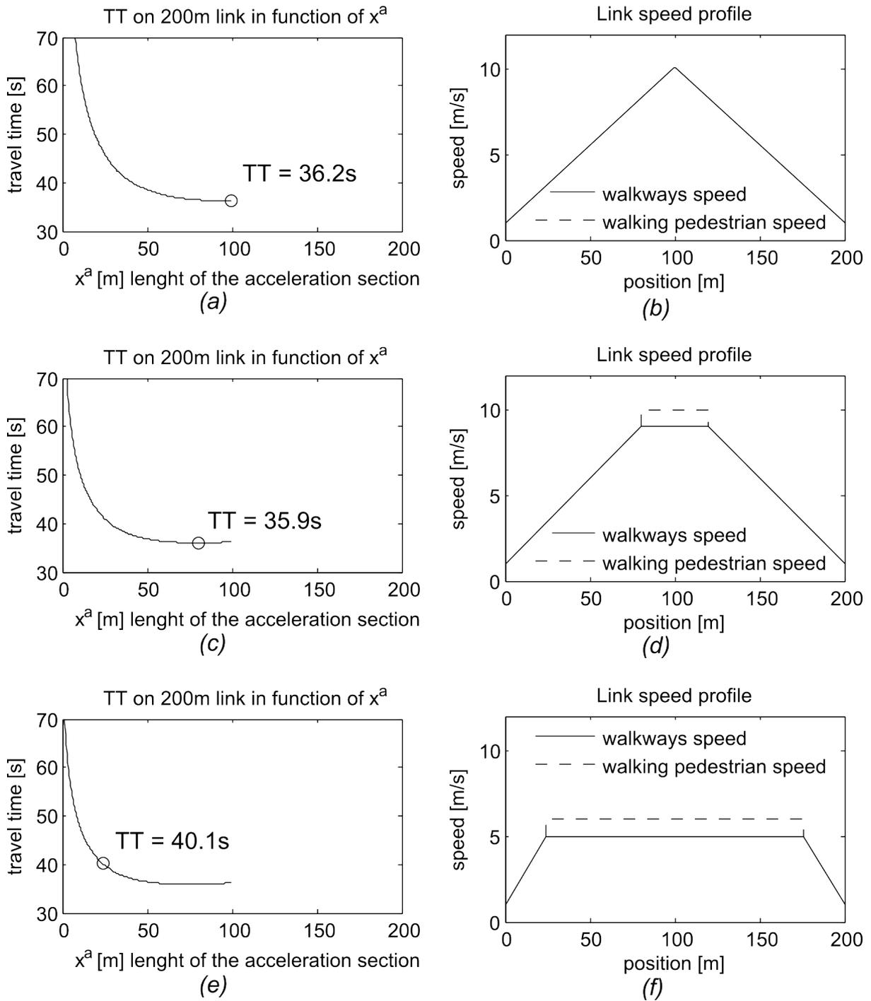
Figure 6: Objective function (left column) and resulting optimal speed profile (right column) in different scenarios. (a) and (b) no pedestrian walking and no constraint  $v^{\max}$ , (c) and (d) pedestrian walking at  $v^w$  and no constraint  $v^{\max}$ , (e) and (f) pedestrian walking at  $v^w$  and constraint  $v^{\max}$ .
