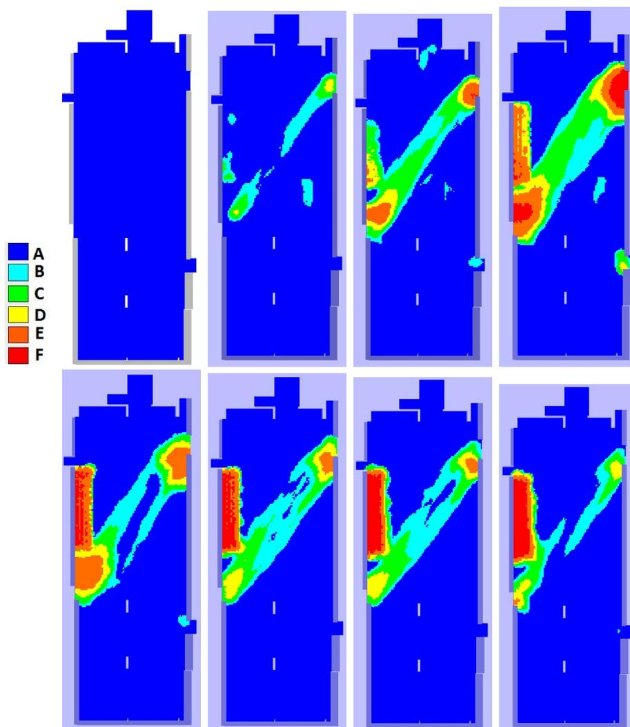
Figure 10: LOS for the first scenario based on HCM standards. On the top left is the first 15-minute interval and on the bottom right is the last 15-minute interval
