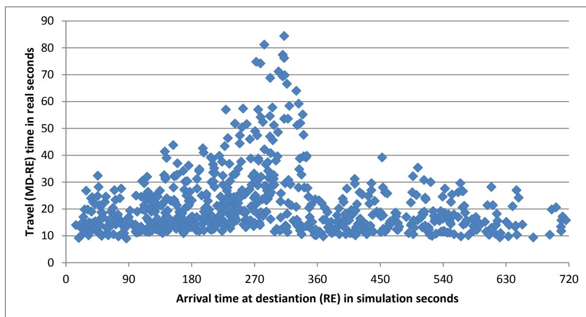
Figure 9: Pedestrians' travel times from MD to RE during simulation (scenario 1)
