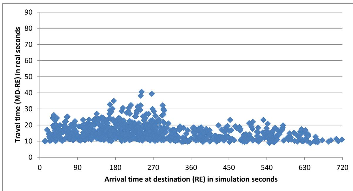
Figure 11: Pedestrians' travel times from MD to RE during simulation (scenario 2)
