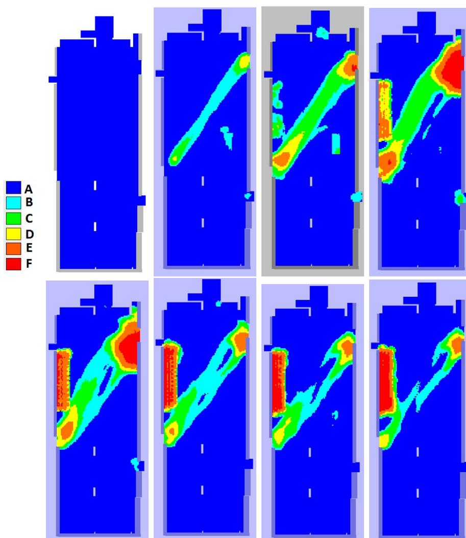
Figure 14: LOS for the third scenario based on HCM standards. On the top left is the first 15-minute interval and on the bottom right is the last 15-minute interval
