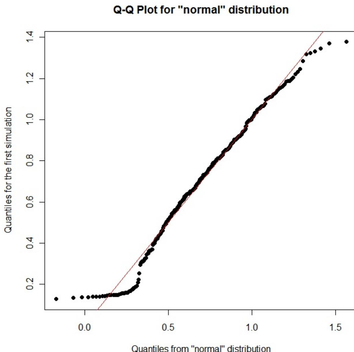
Figure 8: The normality test for the speed results of the first run with default parameter values through quantile-quantile plot
