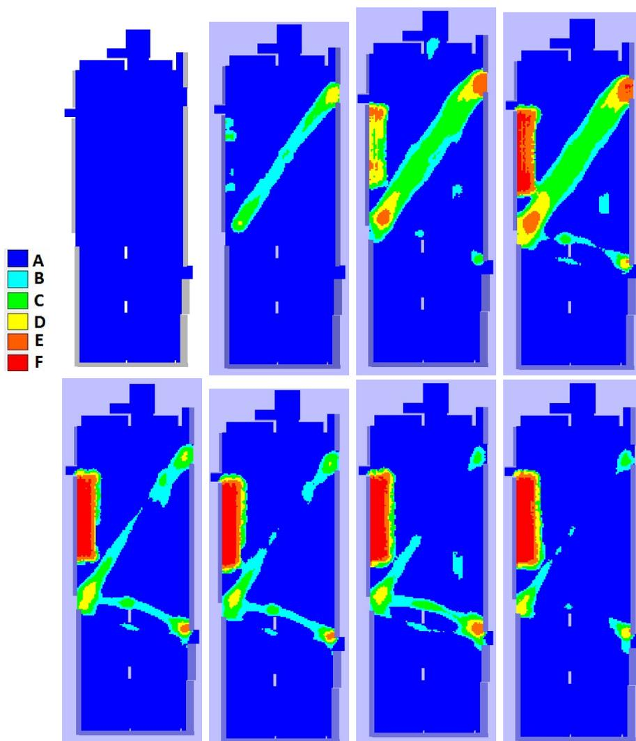
Figure 12: LOS for the second scenario based on HCM standards. On the top left is the first 15-minute interval and on the bottom right is the last 15-minute interval
