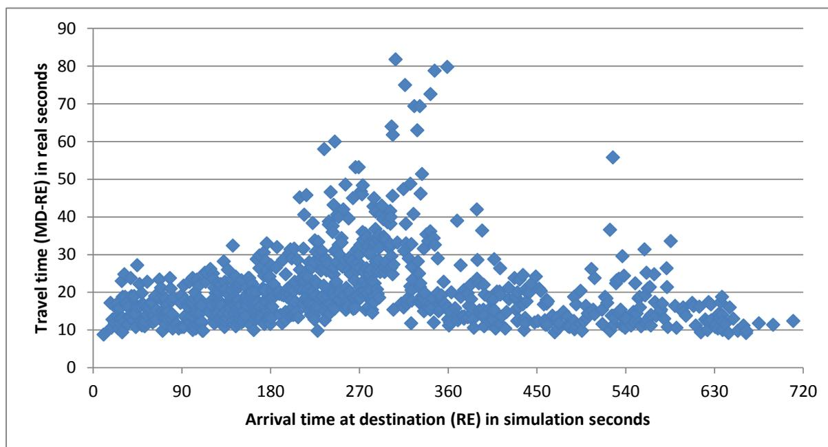
Figure 13: Pedestrians' travel times from MD to RE during simulation (scenario 3)
