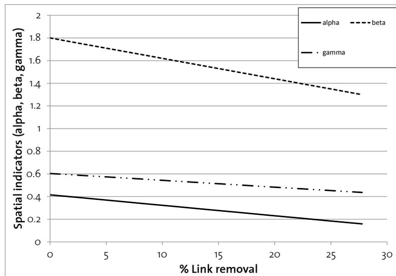
The three indicators present a linear relationship with the link removal for our grid model since the number of nodes is not changed in any scenario (see equations (4), (5), (6)). These indicators are inversely proportional to the link removal (i.e. the indicators decrease as the number of removed links increases, indicating lower connectivity).
