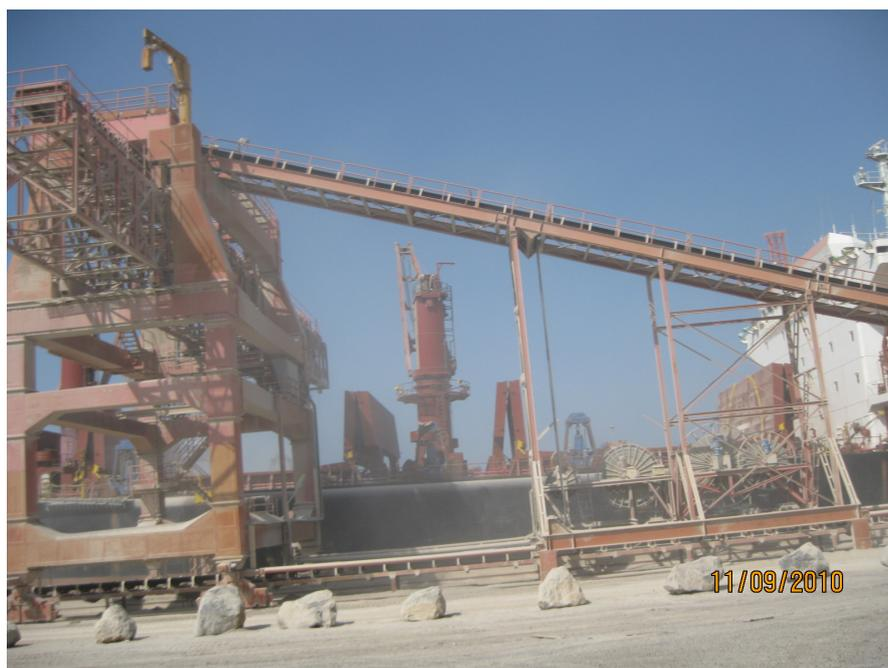
Figure 10: *Rock conveyor at berth 5 at SAQR.*
