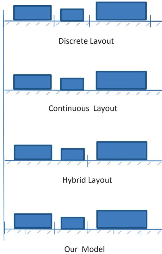
Figure 12: *Different discretizations for berth layout.*
