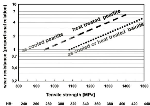
Source: High strength rail steels The importance of material properties in contact mechanics problems Peter Pointer wear 265 (2008) pp.1373-1379
