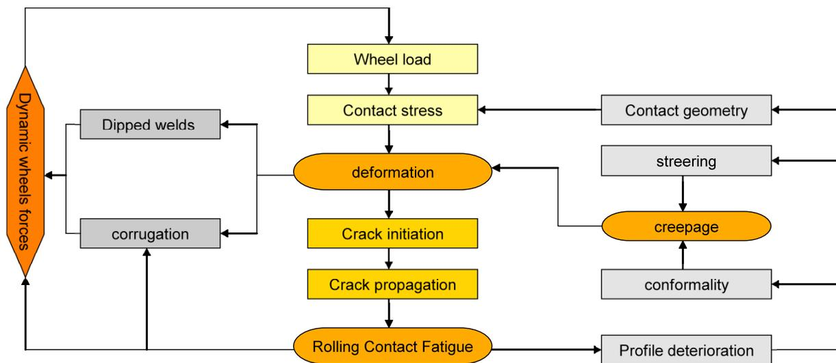
Source: The application of contact mechanics to rail profile and design Eric E.Magel, Joseph Kalousek Wear 253 (2002) p.315
