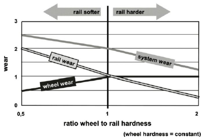
Source: High strength rail steels The importance of material properties in contact mechanics problems Peter Pointer, Wear 265 (2008) pp.1373-1379
