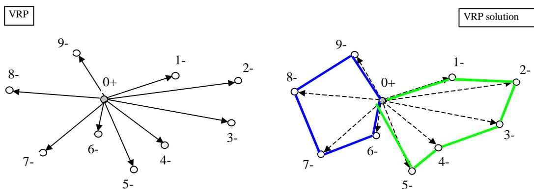
The VRPPD is called a 'Vehicle Routing Problem' (VRP) if either all pickup-nodes or all delivery-nodes are located at a common vehicle location (central hub, depository-node); i.e. either goods or persons are distributed by the depository ( $0^+$ ) on the certain final destinations (Fig. 3), or they are loaded at their respective origin place and transported to the depository ( $0^-$ ).
