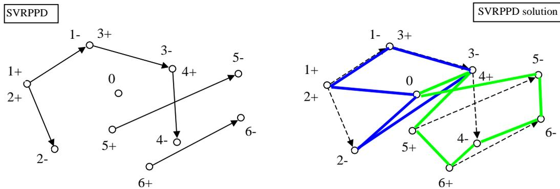
At the 'Standard Pickup and Delivery Problem' (SVRPPD) every route also starts and ends at the vehicle location (0) but the pickup- and delivery nodes can be put arbitrarily (Fig. 4). Another generalisation of this problem structure leads to the 'General Pickup and Delivery Problem' (GVRPPD) where the vehicles are available in arbitrary places (Fig. 5). The central node (0) serves now as a virtual location for forwarding agency vehicles which can be used at additional vehicle need.
