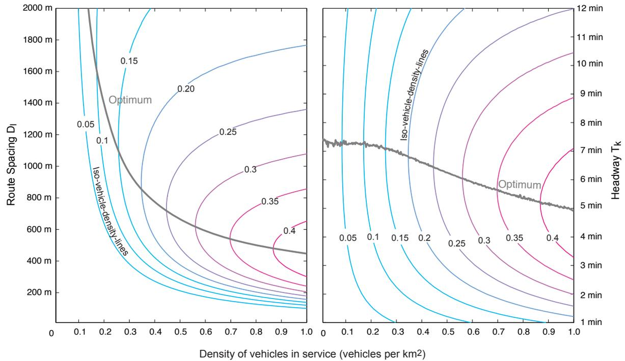
The optimal value for headway does not exceed a certain maximal value (in the example here ~7.5 min). This results also from Figure 8, where optimal headway is plotted against optimal route spacing for varying vehicle densities. Furthermore, Figure 8 shows the optimal values for stop spacing that varies only in a small range from 500 m to 650 m.
