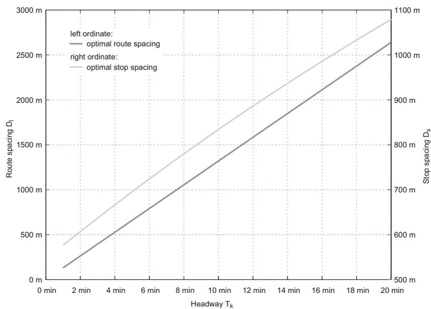
The values obtained in this optimisation for stop spacing are pretty high compared to the values found in practise. Average stop spacing for tram- und bus lines in the city of Zurich are about 350 m. A case study for the tramway network of Den Haag has shown, that stop spacing
