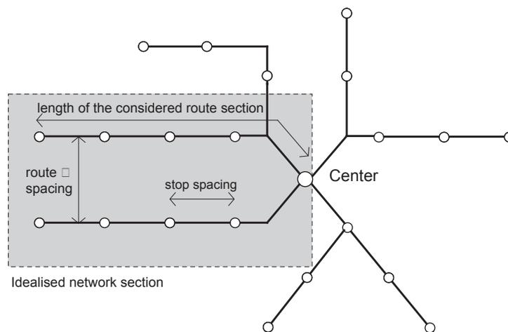
The network design variables have constant values within the idealised network section. This allows determining supply quality analytically within the section.
