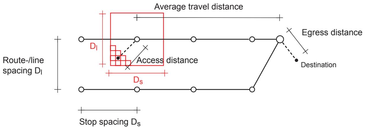
To get optimal values for the network design variables stop spacing, route spacing and headway the maximum in share of public transport usage in dependency of these network design variables is calculated by searching the null of the corresponding function (function (18)).
