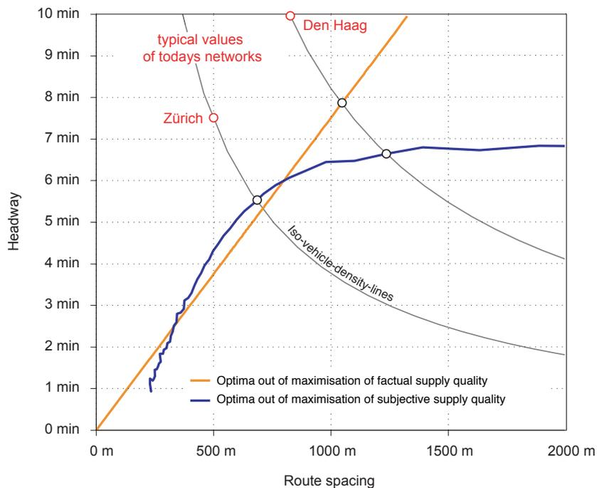
Below a specific supply density attractiveness of public transport is higher when its supply is concentrated on corridors with high demand, where frequencies remain on the required high level. In exchange, the development of corridors with lower demand should be abandoned.
