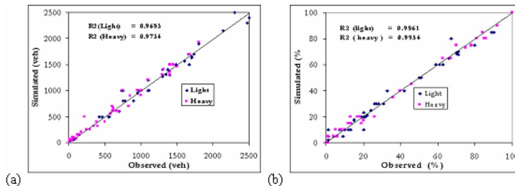
Figure 5 **Observed versus Simulated queue volume (pcu)**
