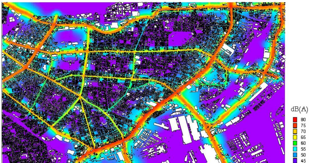
Figure 7 Contour Map when HV is ban along highway route (A ↔ B) (CASE-1)
