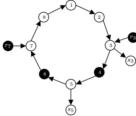
For example, by considering the ring road network of Fig. 2(a) and employing Theorem 4, one can define  $V_O = \{r_3, 4, 6, r_7\}$  as the smallest sets of control nodes, that ensures the system's strong structural controllability. This is illustrated in Fig. 3.
