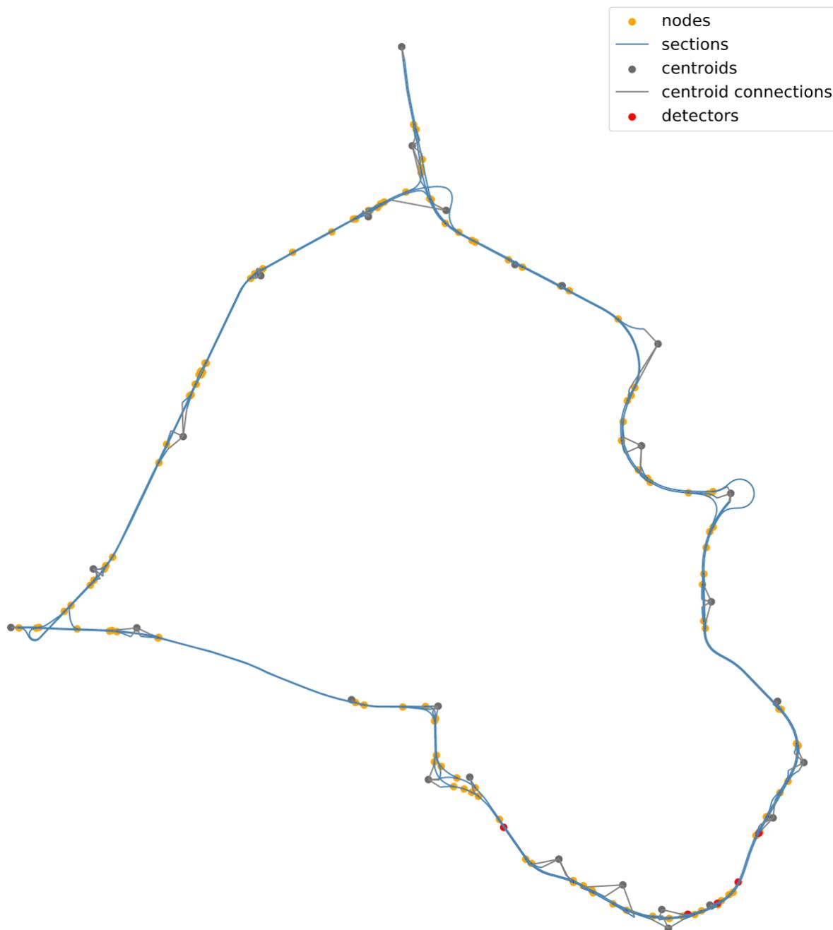
loaded and calibrated in Aimsun microsimulation software. The base scenario demand utilizes traffic counts from morning peak hours. The Origin-Destination (OD) matrix has been derived within Aimsun software from static OD adjustment by using Frank and Wolfe algorithm.
