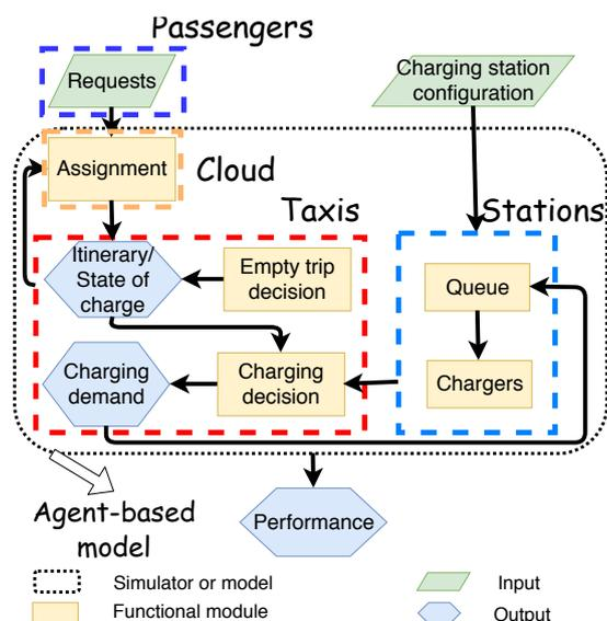
**Figure 1:** Agent-based charging station performance model
