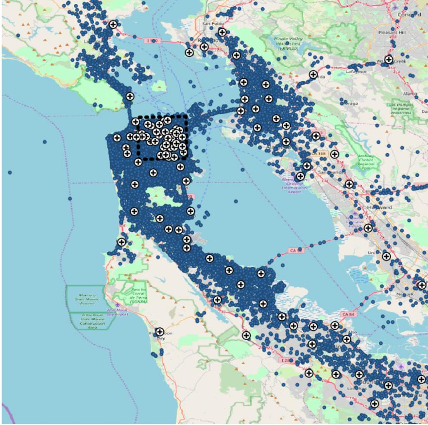
**Figure 3:** The potential 100 locations of charging station, represented by the circles with cross
