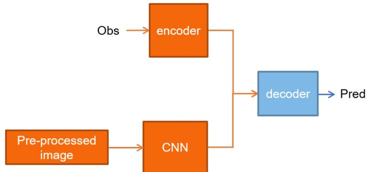
layers for the model is chosen as 128 and the embedding dimension is 64. The CNN network consists of 2 2-dimensional convolutions with kernel size of 8, stride of 4 and output channels of 16 and 32. The convolutions are followed by a 128 node fully connected layer.
