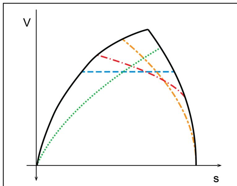
The black line represents the minimal running time for a given case. This strategy illustrates the maximum energy consumption<sup>2</sup>. The different colours represent different strategies, how to reduce the maximum energy consumption:
