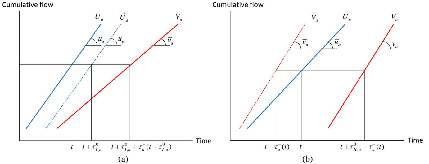
Now assume that the link is either in a spillback or a congested state for which holds that  $\bar{u}_a \leq \bar{v}_a$ . Then we can write  $\tau_a(t) = \tau_{ll,a}^0 - \tau_a^-(t)$ , where stationary maximum (hypercritical) travel time  $\tau_{ll,a}^0$  and (time-dependent) time saving  $\tau_a^-(t)$  are defined through
