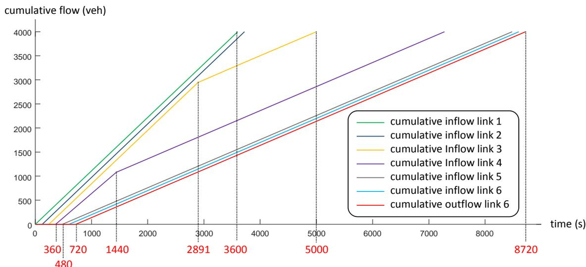
Figure 3: Residual queues in static model on the corridor network
