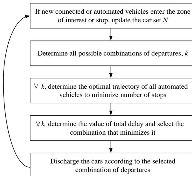
Figure 2. Flow chart of the algorithm
