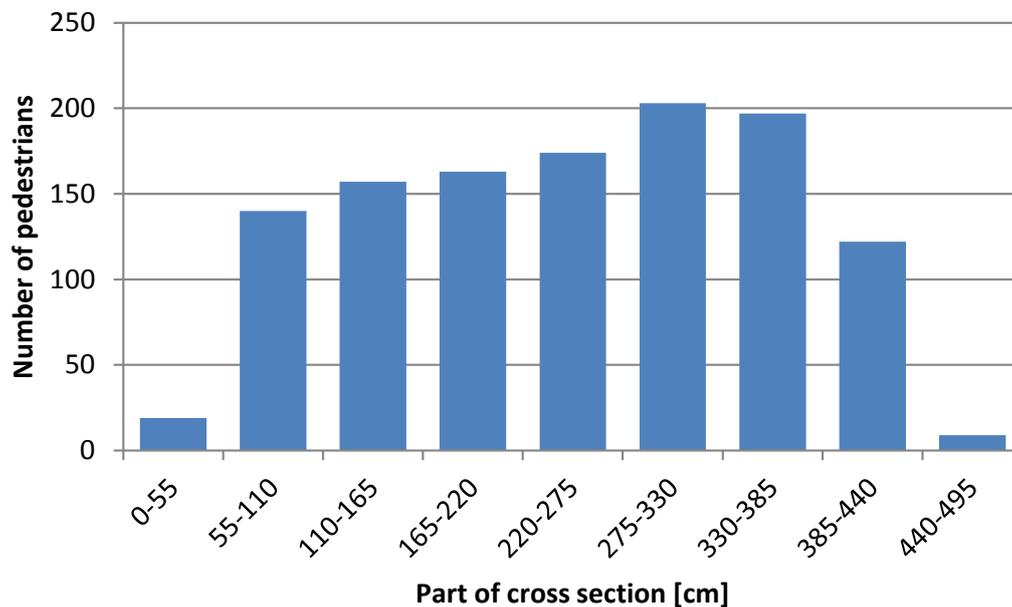
to maximize their mutual distances within the boundaries of the cross section. For example, when two pedestrians cross the measurement area at the same time they typically keep one or two lanes between them. This effect is increased by the more heterogeneous characteristics of commuters compared to a uniform group of pedestrians like students. They are expected to exhibit larger speed differences resulting in overtaking, during which a distance has to be observed in order not to impede others.
