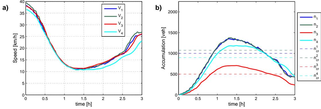
Figure 5: Results from the developed DTA model a. speed evolution, b. accumulation evolution
