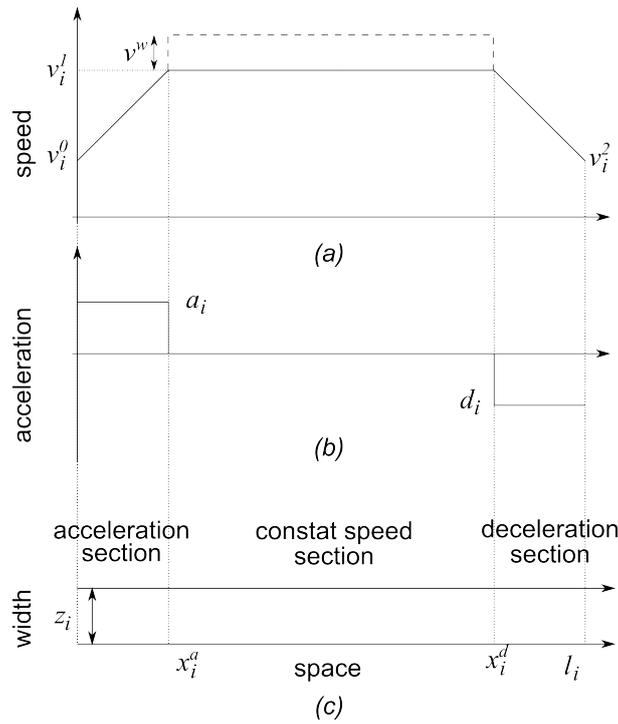
Figure 3: Accelerated moving walkway characteristics. (a) speed profile, (b) acceleration profile and (c) width profile over space of a standard AMW.
