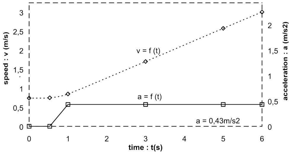
Figure 4: Complete speed profile of an accelerated moving walkway. Adapted from (Boissac and Cote, 2001).
