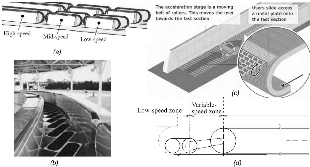
Figure 1: Accelerated moving walkway types. (a) in-line belts, (b) sliding parallelograms, (c) accelerating/decelerating rollers and (d) sliding pallets.
