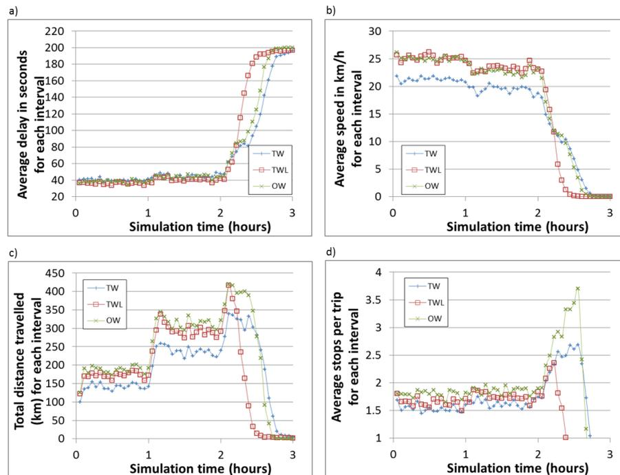
Figure 8. Network performance indicators for TW, TWL, and OW networks considering a higher demand profile (levels of 1.2 – 2 – 2.8).
