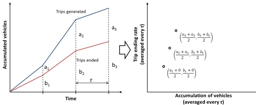
Figure 3. Example of how we obtain the MFD from the accumulation vehicle curves.
