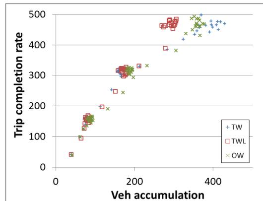
Figure 5. MFDs for TW, TWL, and OW networks in the final iteration, 350, 350, and 112 respectively.
