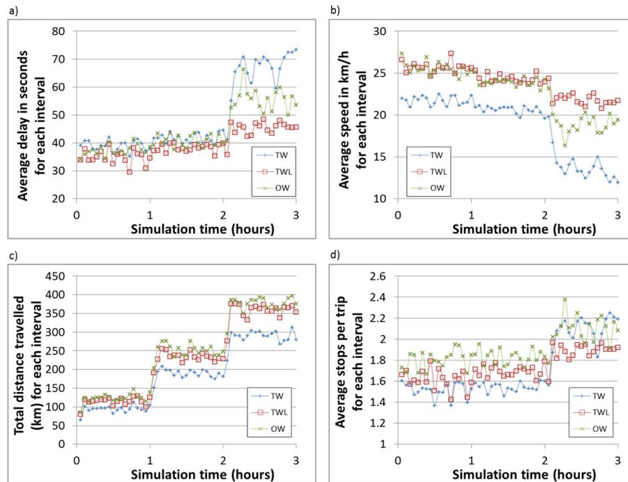
Figure 6. Other network performance indicators for TW, TWL, and OW networks in the final iteration, 350, 350, and 112 respectively.
