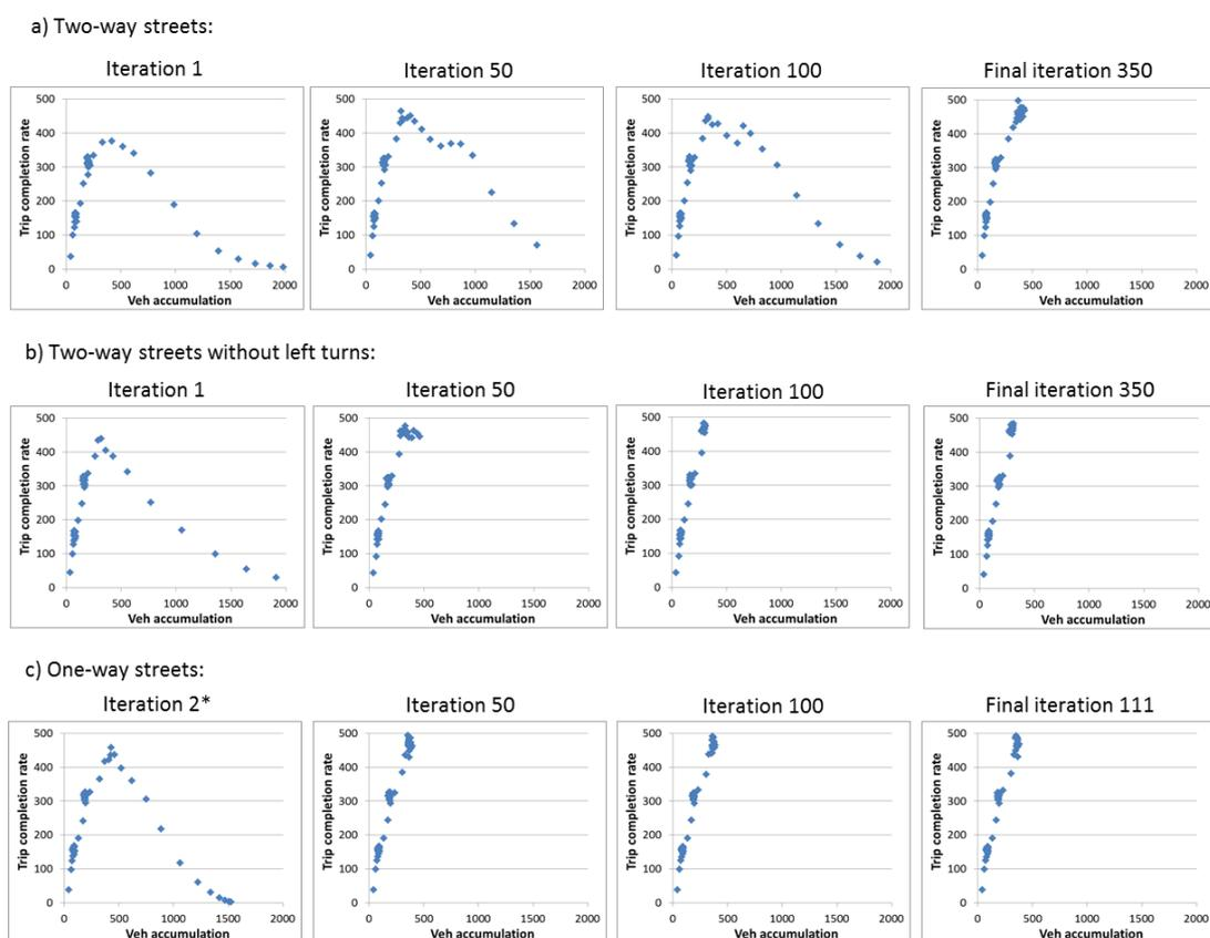
Figure 4. MFDs generated for a) TW, b) TWL, and c) OW networks, and at different iterations of the convergence process.
