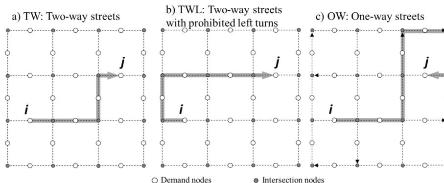
Figure 1. The three networks and their routing options (Ortigosa et al., 2014)
