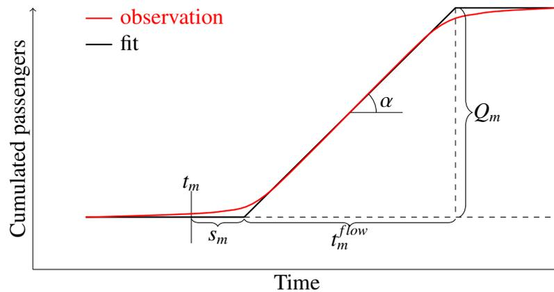
Figure 3: Definition of the parameters used in the piecewise linear step function. Each train induces flows (red curve) which can be modelled by a piecewise linear model (black)
