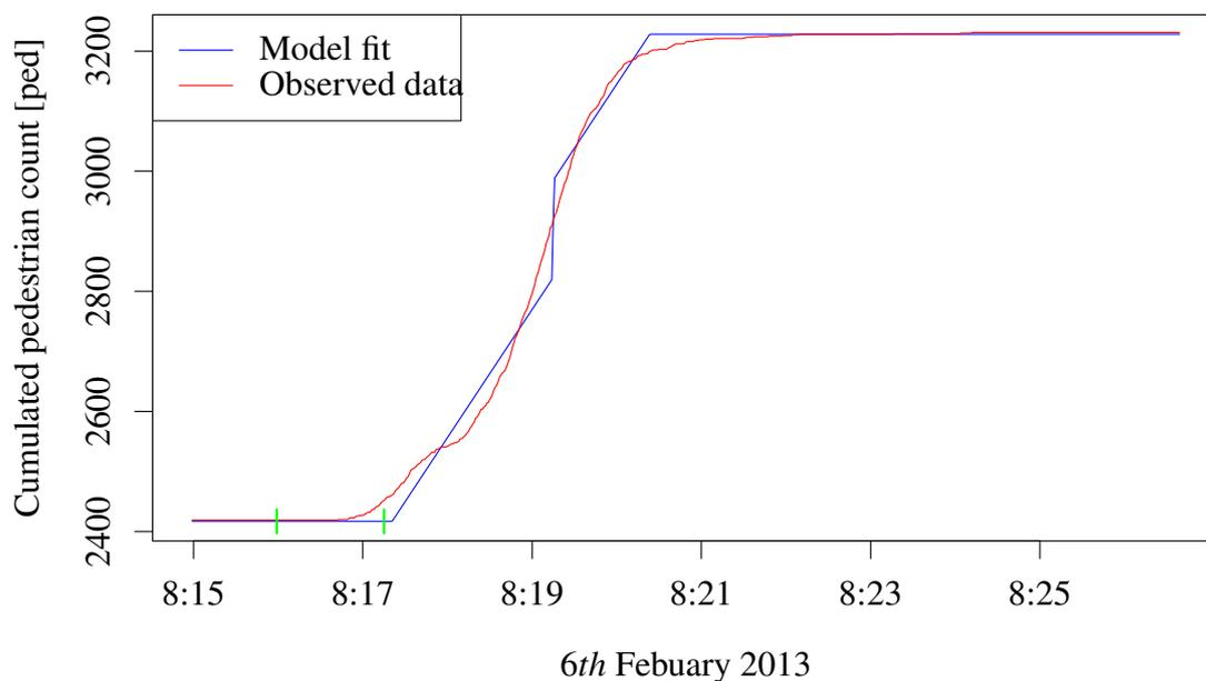
(b) When two trains arrive at the same time on two adjacent tracks, distinction between flows from each train is impossible. At least one of the estimated values of the unloading flow capacity is unrealistic. The number of disembarking passengers must be considered together and only then do the values make sense.
