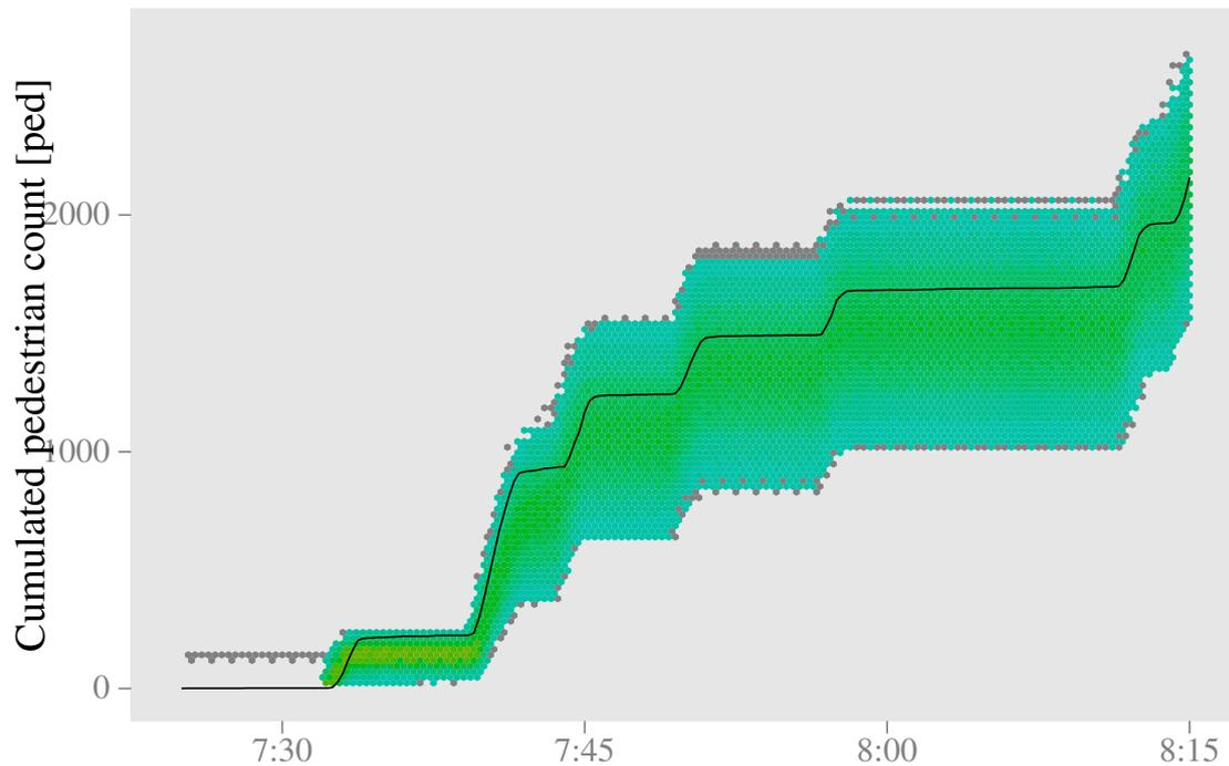
Figure 12: Prediction accomplished for platform 5/6 based on the estimates and the travel survey data. The black line is the observed cumulated pedestrian count on 30<sup>th</sup> April 2013. The density based coloured band is obtained by running the prediction framework many times. The colour scale is logarithmic. This prediction is good and both the estimated shape parameters and the travel survey data prove to be reliable.
