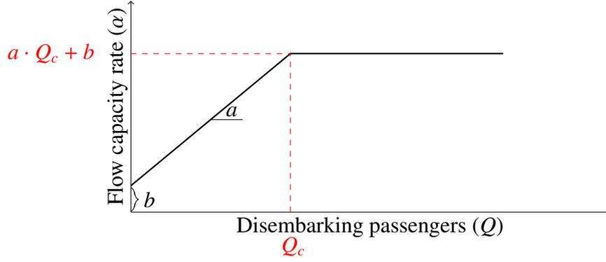
Figure 6: Definition of the parameters used in the model for the flow capacity rate. The assumption is made that the flow capacity rate is linear until an upper limit is reached corresponding to the facilities limits.
