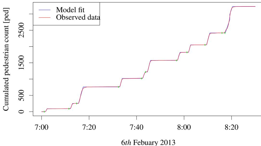
(a) Overall comparison of the fit between the model and recorded data. Discernible differences only appear at the start and end of flows from platforms.
