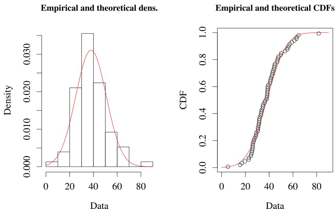
Figure 5: Distribution of the dead time parameter  $s$ . The values of  $s$  are fitted to a normal distribution mean  $=30.2s$  and sd  $=12.8s$ . Using a stochastic model allows sampling from the specified normal distribution.
