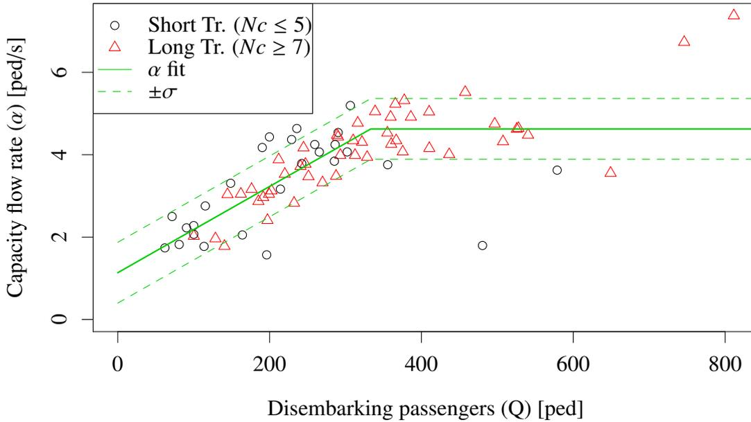
Figure 7:  $Q$ - $\alpha$  plot with the fit of the flow capacity rate model to the data points using least squares. With such a model it is possible to sample within the boundaries in order to obtain an estimation of the disembarking flow capacity rate. Red and black data points indicate the train length, until the turning point  $Q_c$  no trend stands out, and after this point mainly long trains are present.
