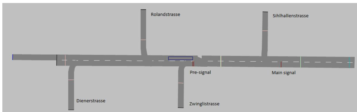
The pre-signal is constructed with two separate signals which together have the same effect as the implemented pre-signal. One signal is a normal signal which is 7 seconds in advance of the main signal. The other signal is a bus actuated signal which turns red for 12 seconds whenever a bus is detected before the pre-signal. These two signals are placed closely
