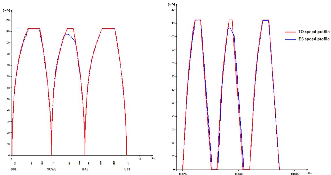
Results from simulation, in terms of energy spent with Energy Saving speed profile and with Time Optimal speed profile are shown in figure 5.
