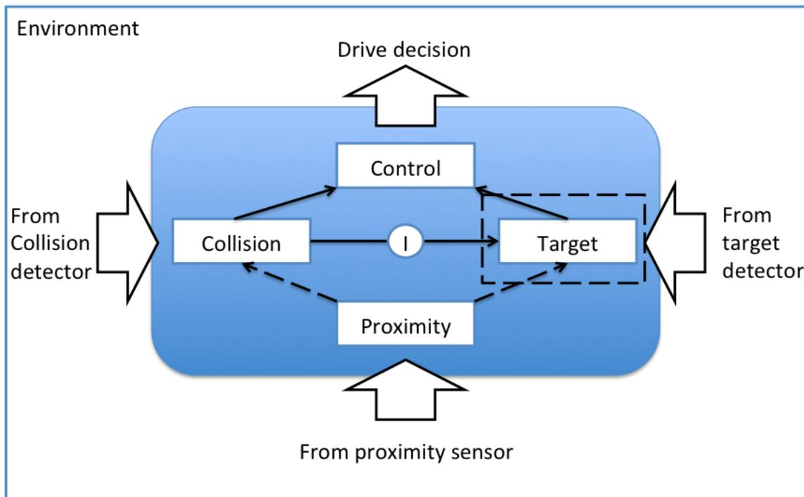
detect the adjacent distances and collision status then pass them to the next blocks, while the target layer and the control layer need to process all the inputs and then decide which control measures to take. These two layers apply Hebbian learning, over time, the weights will pick up the patterns (or correlations) of the collision layer and the control measures. And those with strong correlations will be strengthening by assigning higher weights and irrelevant events will be ignored.
