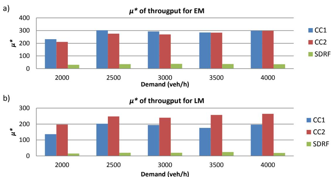
Figure 4 clearly shows that parameters  $CC1$  and  $CC2$  have a much higher  $\mu^*$  than the parameter  $SDRF$  across all scenarios. It indicates that the parameters  $CC1$  and  $CC2$  are more influential than the parameter  $SDRF$ , independently of the adopted merge control scheme and the traffic demand. This also shows that the variance from the safety distance defined in the VISSIM car-following model has a great contribution to the variance of the work zone throughput.
