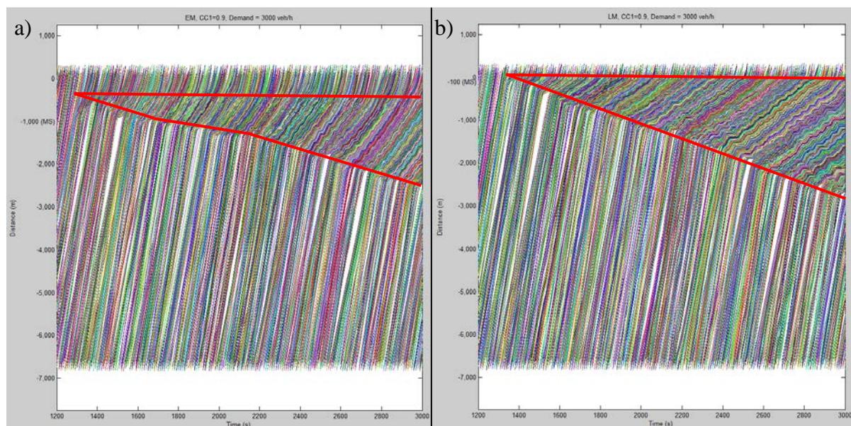
In Figure 6, the formation of the queue also starts earlier in the EM scenario (around 1,310 s) than in the LM scenario (around 1,350 s). However, at the end the queue in the LM scenario (around 5,222 m) is slightly shorter than in the EM scenario (around 5,387 m). Therefore, when  $CCI$  is high, the queue grows slightly faster in the EM scenario (around 3.18 m/s) than in the LM scenario (3.16 m/s).
