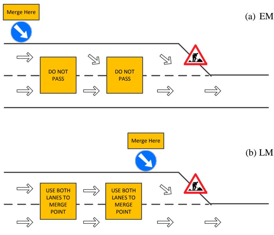
The static EM control (Figure 1a) aims at encouraging drivers to merge as early as possible before they reach the mandatory merging point. The control signs providing the information about the lane drop are placed significantly upstream of the lane drop itself. This control scheme reduces the potential conflicts or frictions among the drivers merging at the last minute. As a result it might reduce the accident rates close to the merge area and guarantee the through flow.
