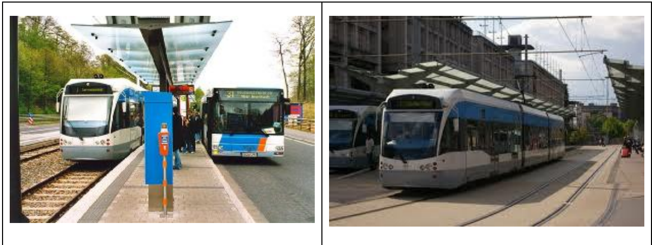
Figure 7: Tram-train system in Saarbrücken, the first low-floor tram-train vehicle
