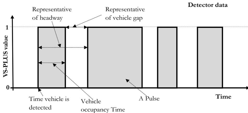
The above filter of minimum occupancy and minimum gap can only remove noise in the pulse. This does not resolve the problem of detector counting error due to closely spaced vehicles, cross-talk etc. For instance, if the gap between vehicles is small and detector is not able to differentiate two consecutive vehicles then a long pulse, instead of two pulses is obtained. This results in undercounting. CUPRITE addresses this issue of detector counting error.
