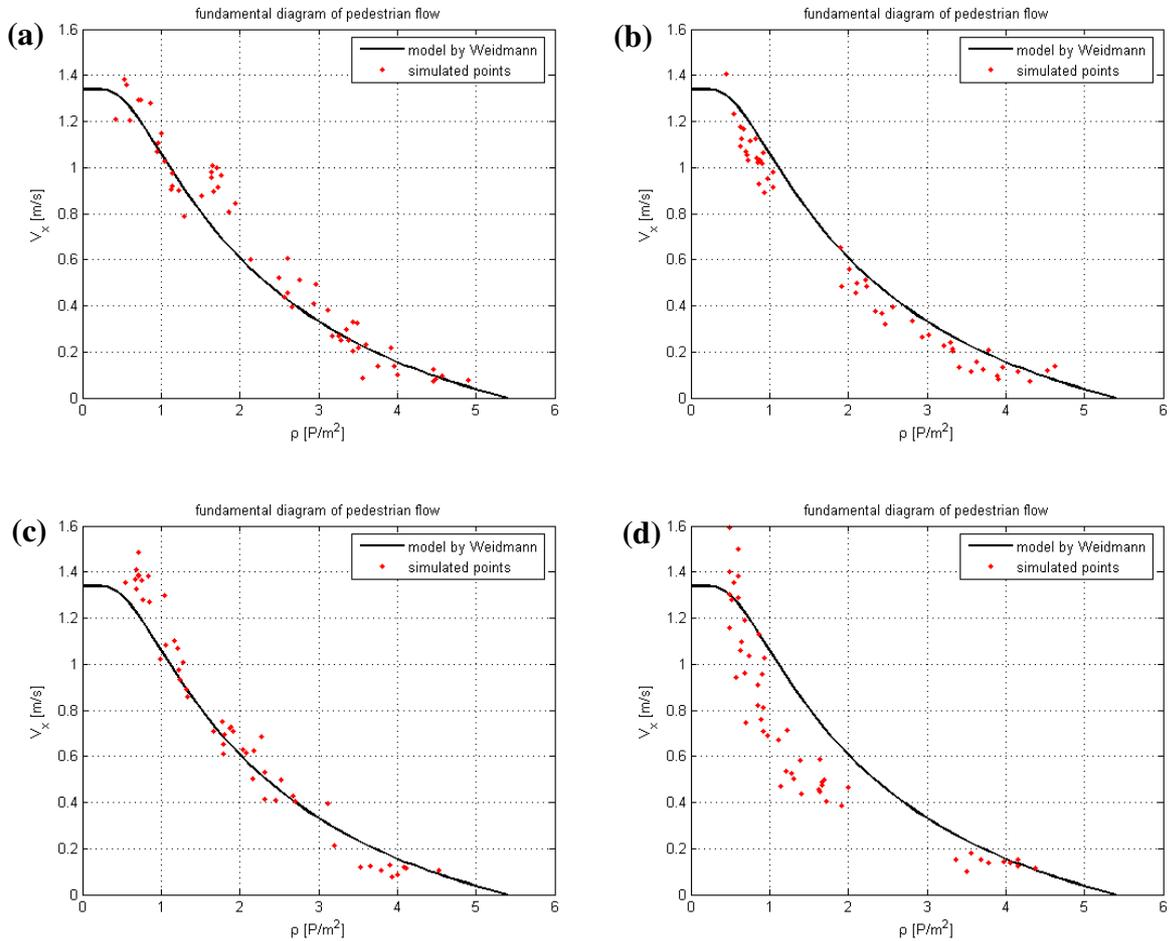
Although we have only 60 data points (red dots) per parameter combination, we see that mainly for (a) and (c), and less for (b) the dots are distributed more or less around the reference curve, whereas for (d) we see large deviations. These qualitative findings are in good accordance with the measures for  $\tilde{g}_{\alpha\beta}$  as shown in Figure 4. From this we can conclude that the macroscopic measure seems to be meaningful for the parameter estimation task in the context herein.
