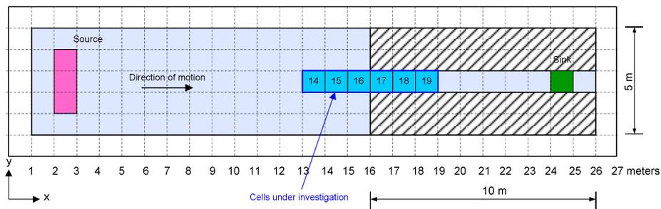
To have densities, that span the greatest possible range within the fundamental diagram, i.e. ideally from 0 to  $\rho_{\max}$ , the pedestrian flow at the source was generated according to Figure 3, where the positions of the pedestrians in the starting area were determined randomly.
