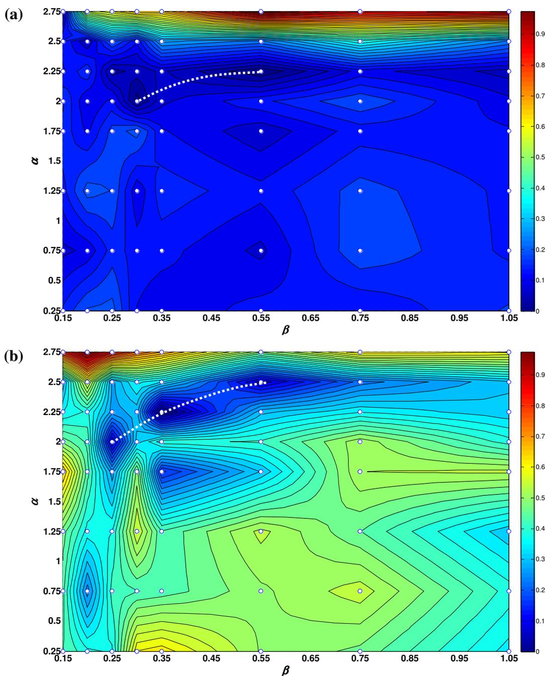
Finally, Figure 9 shows the combined assessment using the average of all cells for the macroscopic contribution. We see a clear minimum for  $\alpha^* = 2.25$  and  $\beta^* = 0.35$ . If we compare these values with those from literature (see section 3.4) we find that  $\alpha^*$  as well as  $\beta^*$  are within the expected range.
