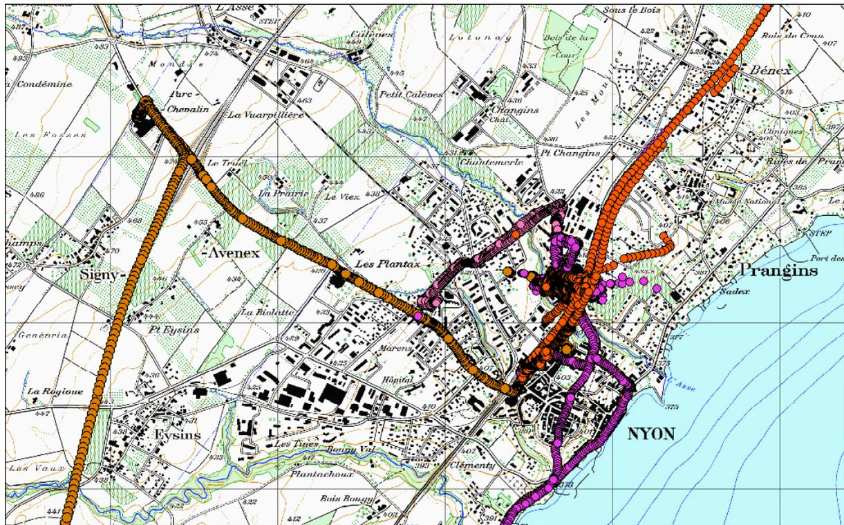
Tracking data includes trips by car (brown and cyan), by train (red) and by bicycle (pink). The large bulk of points in the centre-right results from positioning errors generated while the device was inside my home; a few “one way trips” going out of that bulk are in fact additional measurement errors.
