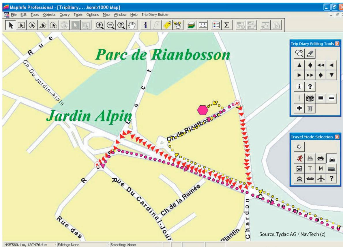
The Trip Diary Editor breaks down raw tracking data into trip segments, delimited either by activity places (stays longer than 90 seconds) or by trip pauses (shorter stops, identified by way of speed variations). In editing mode, trip segments can be displayed one by one, allowing the interviewer to re-enact the respondent's travel diary for primary analysis (verifications, travel mode imputation) and as an input for prompted recall interviews.
