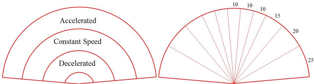
**Fig. 2.** Discretization of the space based on 3 speed regimes and 11 radial directions. The numbers in the figure on the right represent the angles, in degrees, of each direction.
