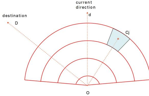
**Fig. 3.** Given a destination  $D$  and the current direction  $d$ , the angles defined by the *direction* and *destination* attributes are respectively  $d\hat{O}Cj$  and  $D\hat{O}Cj$ .
