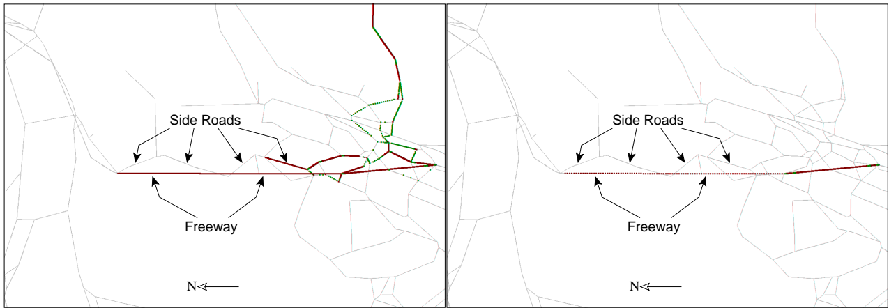
Figure 7: A freeway and side roads with the agent database strategy at 19:00 (left) and 20:00 (right). As with the “max and offset” strategy, the side roads are emptying, while the freeway contains vehicles. This shows the agent database is a solution to the freeway problem.
