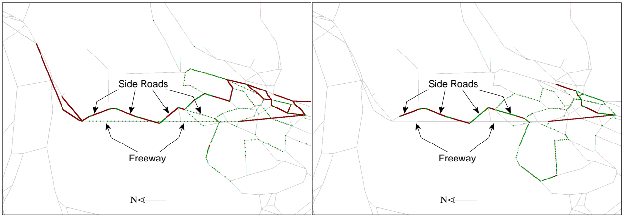
Figure 3: A freeway and side roads with the offset time bins strategy at 19:00 (left) and 20:00 (right). The side roads contain many vehicles while the freeway contains very few or none.
